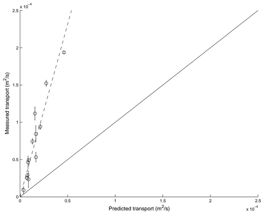
**Figure 3. Comparison between predicted and measured (Dohmen-Janssen et al., 2002) net sediment transport rates in current direction for co-directional sinusoidal waves and currents. Predicted bedload is based on  $k_N = D_{50}$ . The line of perfect**
