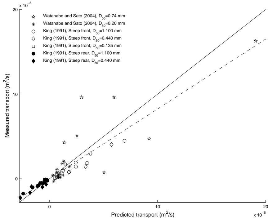
**Figure 2. Comparison between predicted and measured net sediment transport rates for asymmetric, non-skewed waves (no current). Predicted bedload is based on mobile-bed roughness. The solid line corresponds to perfect agreement between predictions and measurement, while the dashed line is the least-squares fit to the data and corresponds to an overprediction by a factor of 1.2.**
