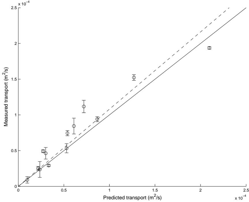
Figure 4. Comparison between predicted and measured (Dohmen-Janssen et al., 2002) net sediment transport rates in current direction for co-directional sinusoidal waves and currents. Predicted bedload is based on mobile-bed roughness. The solid line corresponds to perfect agreement between predictions and measurement, while the dashed line is the least-squares fit to the data and corresponds to an underprediction by a factor of 1.1.
